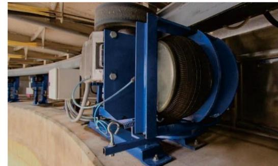
Heavy-duty drive units with automatic adjusting and attaching system
