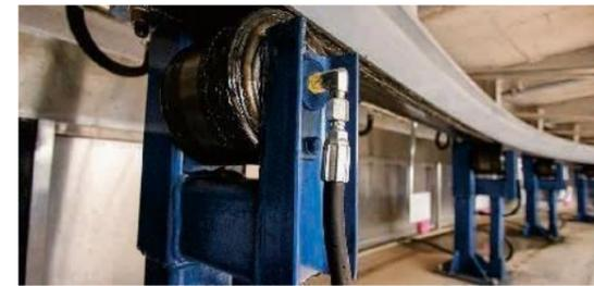
I-beam automatic lubrication system
